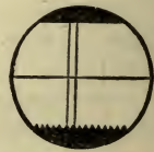
Field of large filar micrometer showing cross hairs and recording comb.
