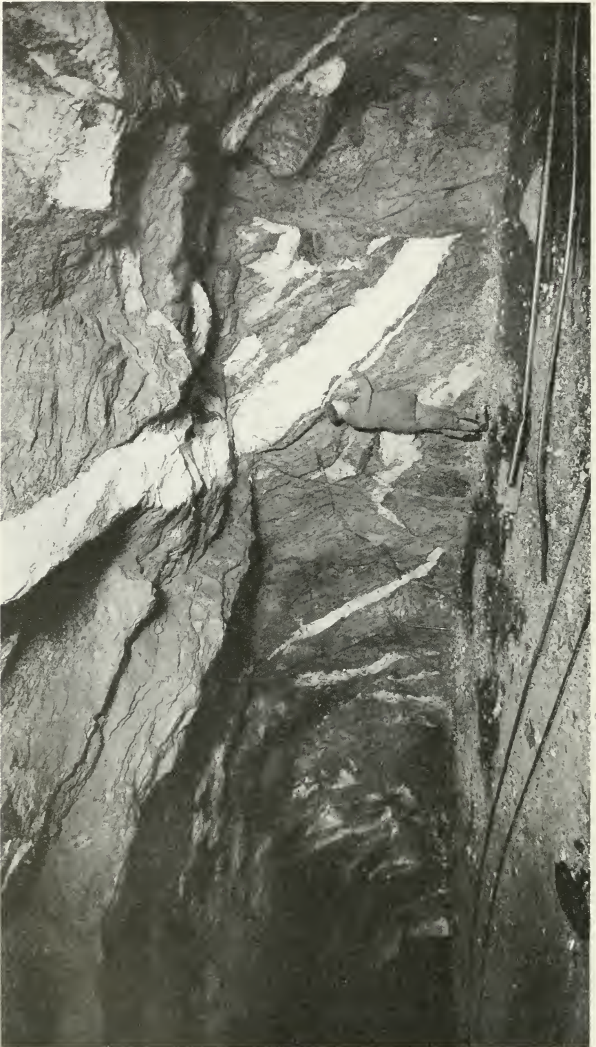
Ore body on 4th level, Dome mine. A fault is indicated at the right side of the illustration
