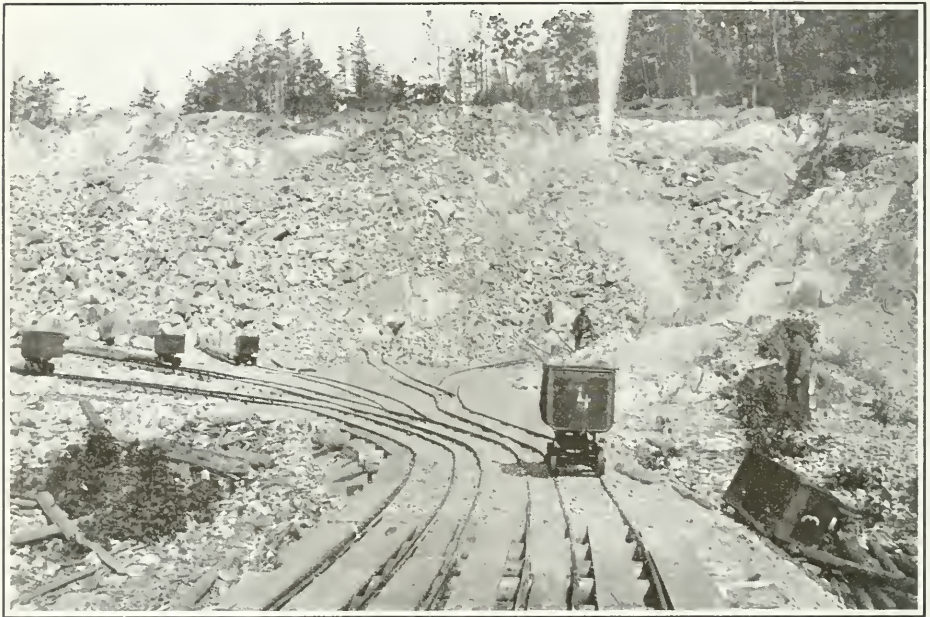
Fig. 8—Quartz quarry near Killarney on the north shore of Lake Huron. The quartz is used for making ferro-silicon
