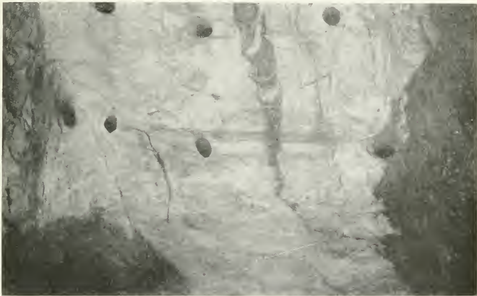
Quartz vein on 100-foot level, Porcupine Crown mine. The dark spots are drill holes
