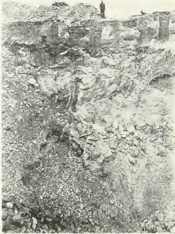
Open pit, Dome mine. The ore body consists of quartz veins irregularly distributed in the schist, and overlain by 6 feet of clay and gravel. Sept., 1914
