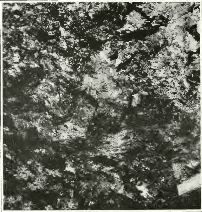
Fig. 16—Residual Kaolin (white spots) in iron ore at Helen mine
