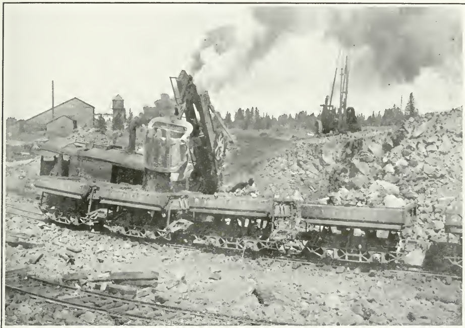
Fig. 13—Steam shovel loading trap rock on cars at the quarry of the Martin International Trap Rock Company, at the town of Bruce Mines, on the north shore of Lake Huron
