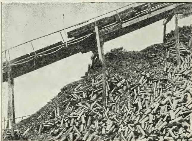
FIG. 28.—The bark sifting down on this pile of pulpwood will hold the moisture from rains and form a splendid incubating medium for the fungi which decay pulp wood. Preventable decay losses in pulp-wood storage yards managed without regard for sanitation amount to over 29,000,000 cubic feet annually
