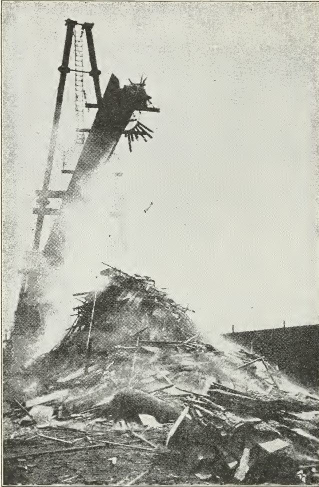
FIG. 17.—In the average sawmill about 45 per cent of the log as it reaches the mill finally goes to the burner in the form of bark, slabs, edgings and trim, saw kerf, and other waste forms. In many mills some of this material is converted into small products or used as fuel, but the potential salvage is enormous
