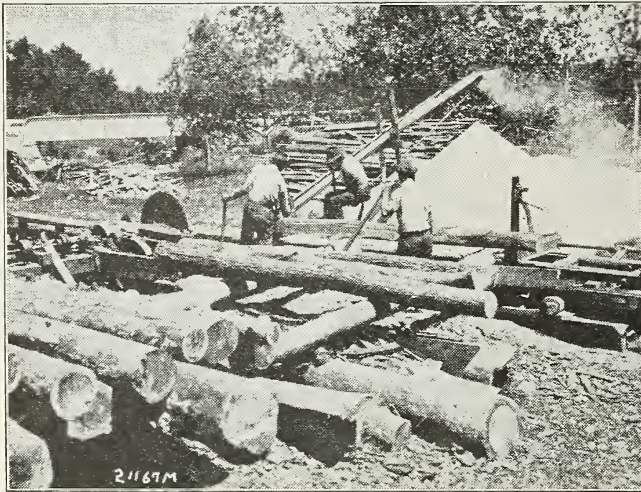
FIG. 23.—Ten per cent of our lumber is now being cut by such mills, with unnecessarily heavy wastage through the use of thick saws and mismanufacture
