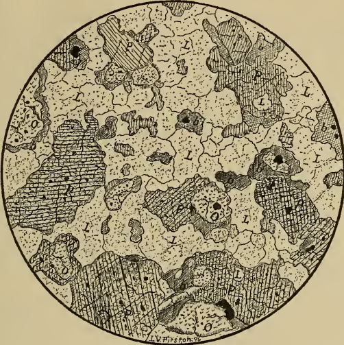
Micro-drawing of Missouriite \times 6 ; P = pyroxene, O = olivine, b = biotite L = leucite.
