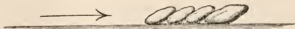
SHOWING THE POSITION ASSUMED BY PEBBLES IN THE BED OF A STREAM.
