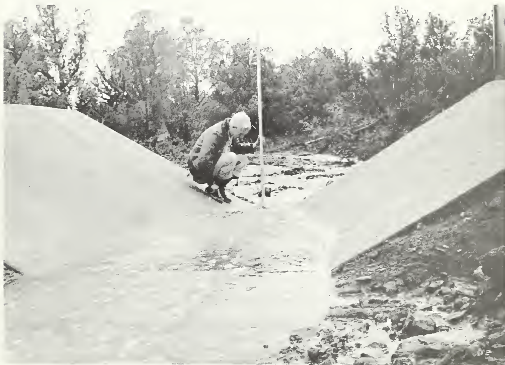
Figure 12. --Flow measurements in a flume on Beaver Creek. The operator is using a velocity head rod to measure water depth and velocity. Flumes of this type are located on 14 small watersheds where various land treatments are underway or planned. To date the flumes have carried discharges up to an estimated 380 cubic feet per second. The flume will measure a wide range of flows and carry large debris loads. Rating of the flume is based on tests in the Colorado State University Hydraulics Laboratory and flow measurements in the field.
