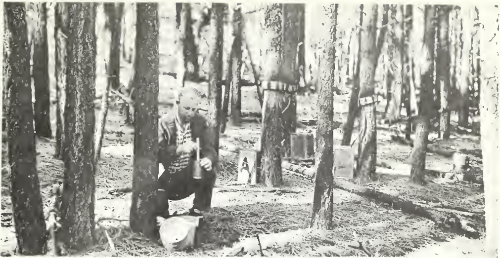
Figure 10. --Measuring rainfall under canopy of pole-sized ponderosa pine. The rain caught in the cans on the forest floor is called "through-fall." Bands around the trees in the center are troughs to catch rain flowing down the trunks (stemflow). In this stand through-fall was 71.4 percent of gross rainfall and stemflow was 8.3 percent. Thus 20.3 percent less rain reached the ground here than in a nearby opening.
