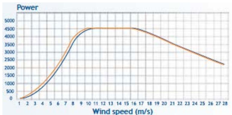
Figure 34. Typical Wind Turbine Power Curve
