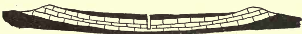
Fig. 40. Conditions for artesian well. A water-bearing stratum lies between two impervious ones, the whole being folded into a trough or syncline. The water falling on the hills at either end runs down the dip and collects at the bottom; when the upper bed is pierced by the well the water is forced up by the pressure of water above and may form a jet above the surface.
