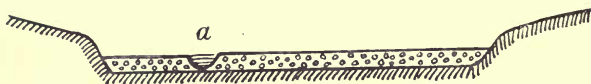
Fig. 25. Cross section of the valley of an old river; a meander plain bounded by bluffs. The dotted portion represents the alluvium formed by the river, which is seen at a , but has at different times occupied every possible position within the limits of the meander belt.
