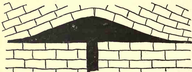
Fig. 4. A laccolith fed by a dyke below; the overlying strata being lifted up to form a dome.
