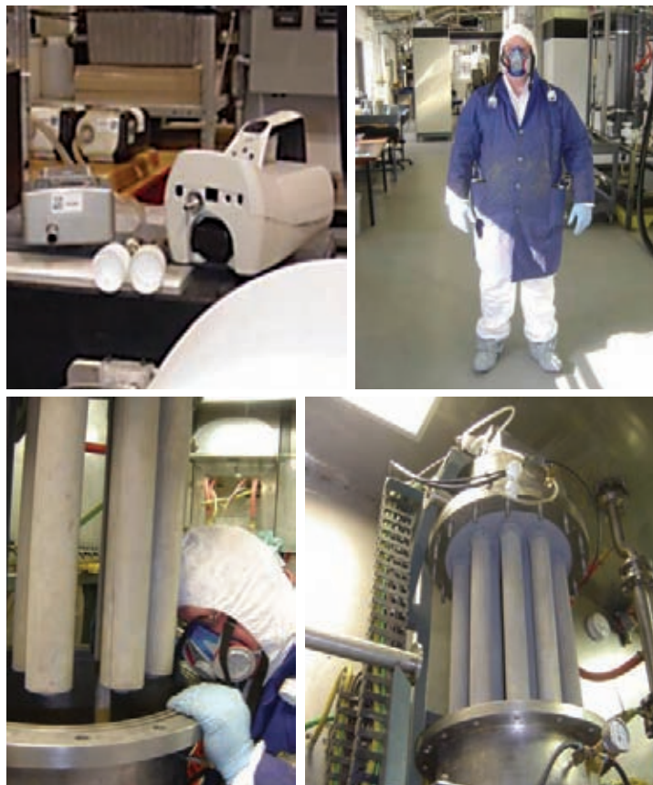
Figure 1. A demonstration of the initial assessment technique with side-by-side sampling using (from left to right) the OPC, co-located open-face filter cassettes, and the CPC: examples of PBZ and source-specific filter-based sampling setup.
