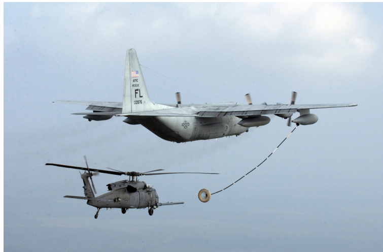
Figure 7: Example of Hose and Drogue
