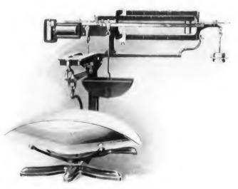
The Board of Trade have examined and tested a pattern of a weighing and counting instrument of 25 lb. capacity, of the form herewith shown, submitted to the Department under the provisions of Section 6 of the above Act, but as the result of the examination was not satisfactory, the Board have declined to issue a certificate of approval.
