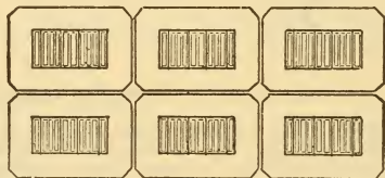
FIG. 48. Cross Section of the Cores and Coils of Three Single-Phase Air-Blast Transformers.
