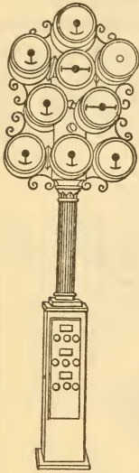
FIG. 34. Post with nine instruments. The three ammeters at the bottom are for a bank of transformers. The six instruments above are for one generator. The plug switches in the base permit testing the calibration of the instruments without removal.
