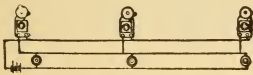
FIG. 39. Three-Line Factory Call. A number of Bells operated by any number of pushes. All bells rung by each push.
