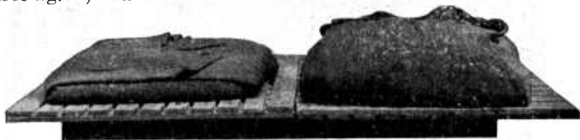
FIG. 4.—Good and bad cheeses. That at the left is uniform in thickness, well covered by the cloth, and will not creep or spread in pressing. That at the right is too thick and will spread out beyond the racks when placed under pressure, making the proper extraction of the juice impossible. The two cheeses were pressed after photographing. The yield from the thin cheese was 64 per cent of the weight of the fruit used and that from the thick cheese 52 per cent.
