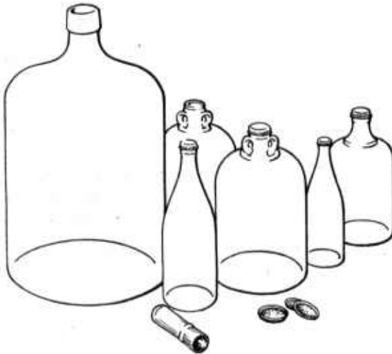
FIG. 7.—Good types of containers. The 5-gallon bottle is a satisfactory storage vessel. It must be sealed with a paraffined cork. The gallon and half-gallon jugs and the pint and quart bottles which are sealed with cork-lined metal caps are good final containers. A satisfactory inexpensive device for applying caps is seen in the foreground of the picture.
