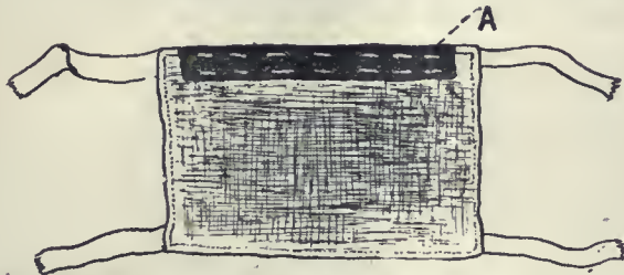
Inside of mask: A, adhesive strip (adhesive surface up) sewed to it.
