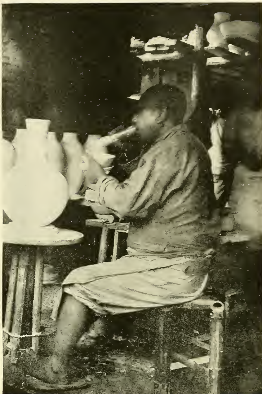
ONE METHOD OF APPLYING PORCELAIN GLAZE
