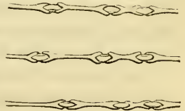
Section of Fir wood (Deal), Longitudinal and perpendicular to the medullary rays; 300 linear.
