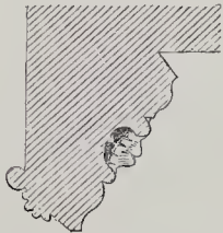
SECTION OF MOULDINGS AT B 3/4 FULL SIZE
