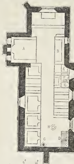
A Sir H. Wilmot's pew. E Clerk's desk. B Clergyman's ditto. F Reading ditto. C Font. G Pulpit. D Staircase to turret. H Stove.
