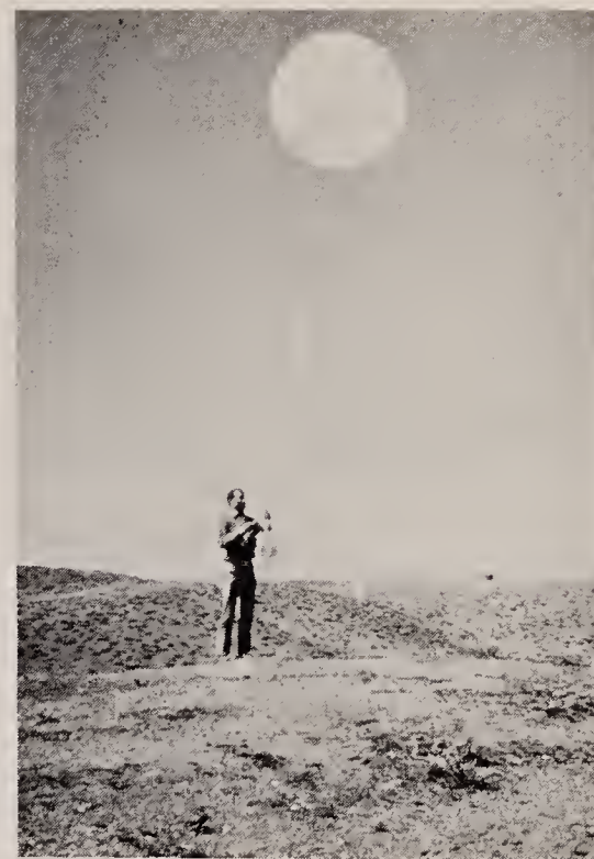
Rawinsonde carries meteorological instruments for air quality studies on the Utah tracts.
