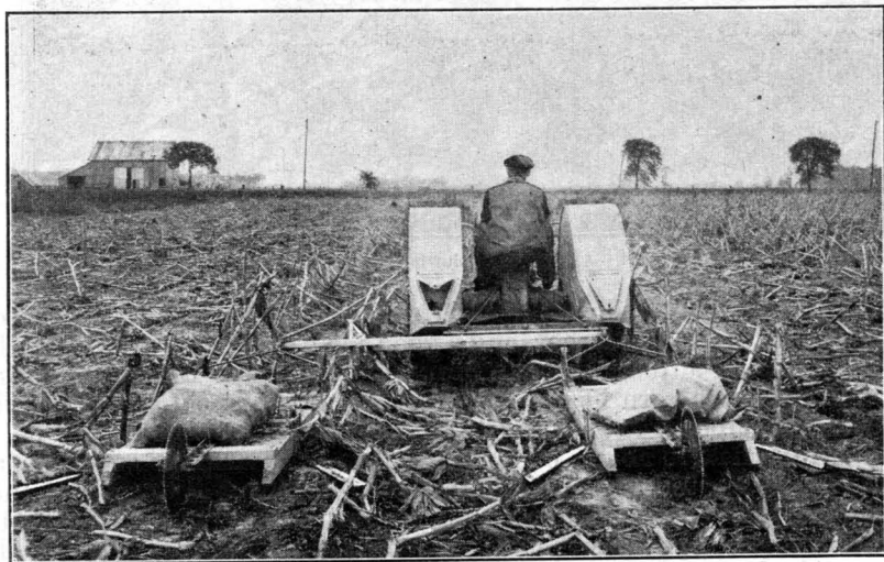
FIGURE 26.—Two sled-type shavers hitched abreast and cutting four rows
