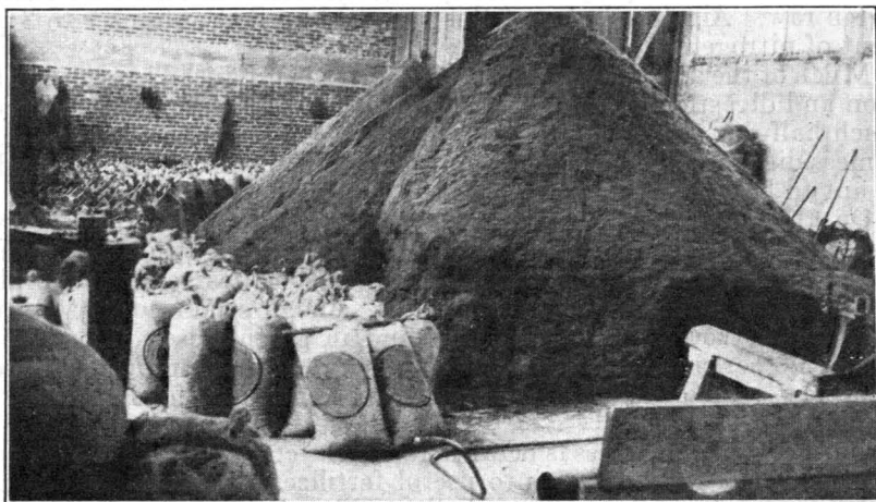
FIGURE 113.—Garbage tankage dried, ground, and screened, when used in mixed fertilizers, furnishes some nitrogen and improves the physical condition and drillability of the mixtures
