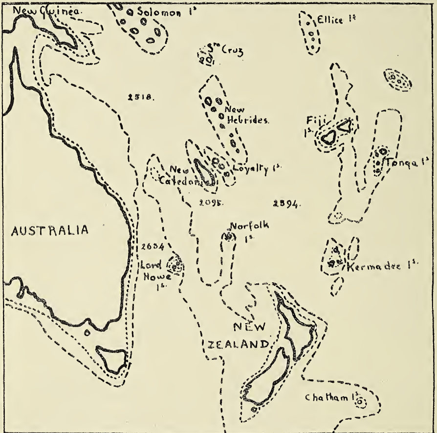
DIAGRAM 3. Soundings in the New Zealand area. ----- 100 fathoms. ..... 1,000 fathoms. Numbers inserted here and there give the depth in fathoms at those points.
