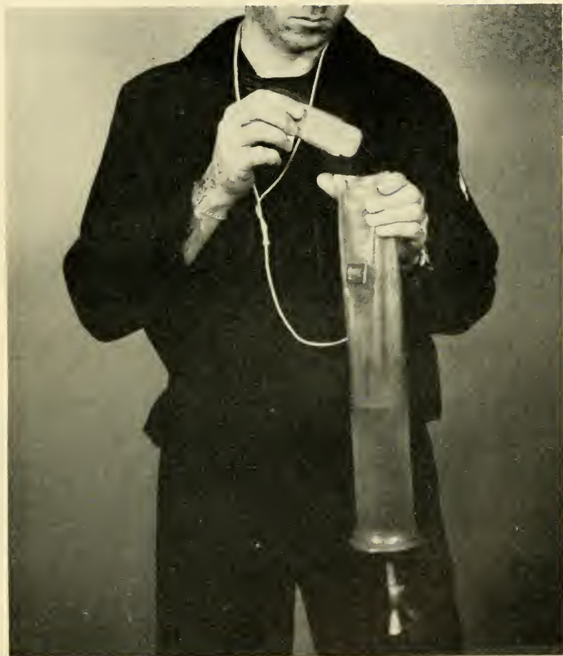
ADDITION OF DESALTING BRIQUET TO PROCESSING BAG CONTAINING SEA WATER.
