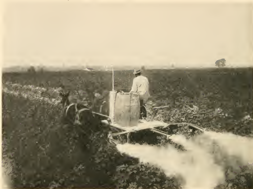
1. AN EARLY-MODEL CART DUSTER DEVELOPED FOR DUSTING COTTON FOR BOLL WEEVIL.
