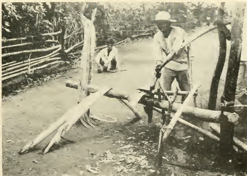
2. STRIPPING ABACA FIBER.
