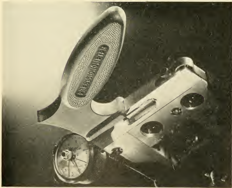
1. AN EXCELLENT EXAMPLE OF METALS-AND-PLASTICS COLLABORATION IS THIS PORTABLE INDICATING COMPARATOR. The handle is injection-molded of Tenite plastic, whose low thermal conductivity prevents the heat of the operator's hand from affecting the precision of the metal measuring components. Courtesy Tennessee Eastman Corp.)
