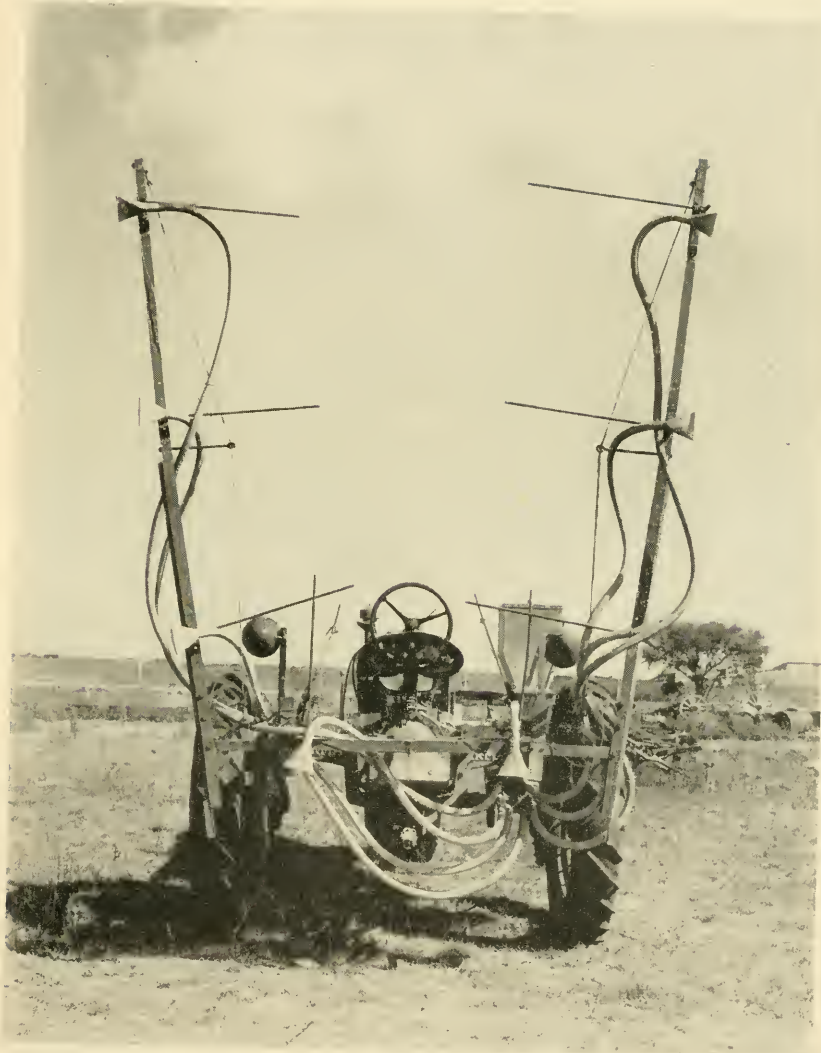
TRACTOR DUSTER WITH EIGHT NOZZLES, WITH BOOMS FOLDED FOR PASSING THROUGH GATES.
