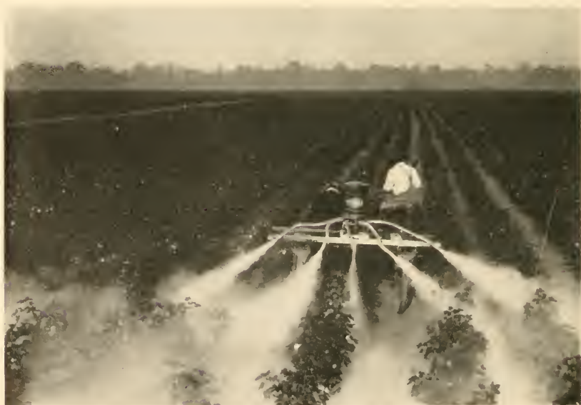
2. A FIVE-NOZZLE POWER-OPERATED CART DUSTER.
