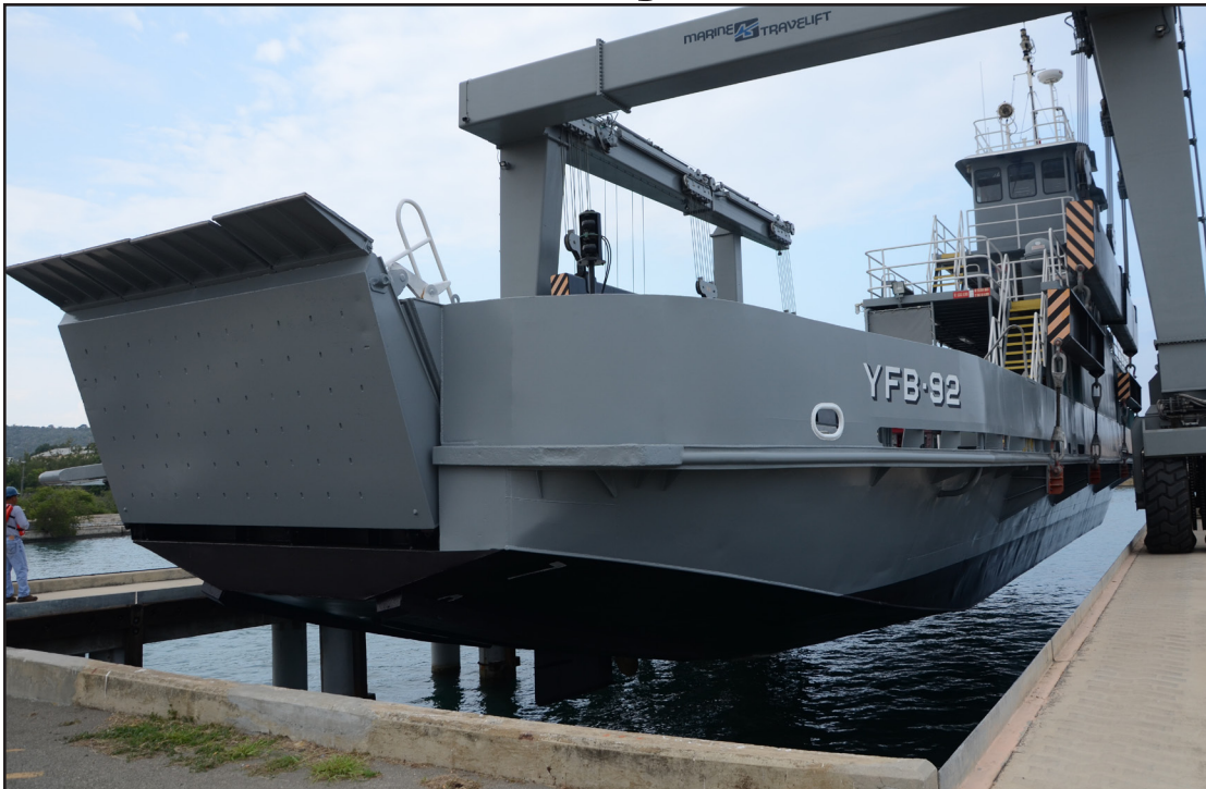
Naval Station Guantanamo Bay's Munilla Construction Management (MCM) branch uses a Marine Travelift to place the newly overhauled ferry back in the water, Mar. 22.
