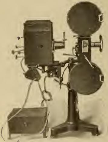
There are 16 pictures to every foot of film, therefore in 4,000,000 ft. the intermittent movement must operate 64,000,000 times. One fourth of a revolution of the intermittent sprocket moves the film the length of one picture; therefore one complete revolution would draw down four pictures and to move the above amount of film, would require 16,000,000 complete revolutions.
