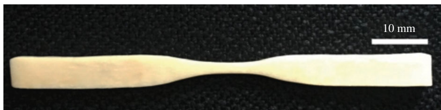
Figure 8. Example dog-bone preparation for mechanical testing. Scale bar, 10 mm.
