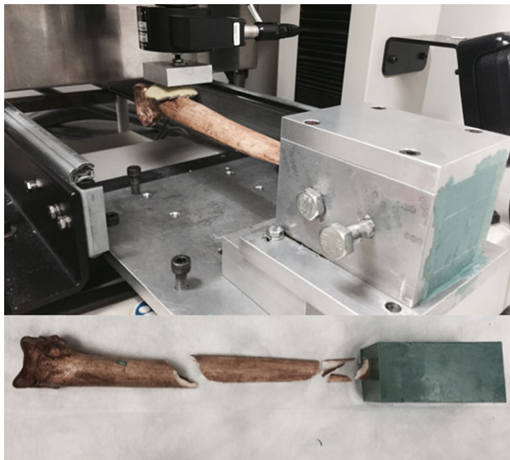
Figure 7. Cantilever bending test configuration; the cassowary bone dagger was fixed at 20% of the overall length from the tip.
