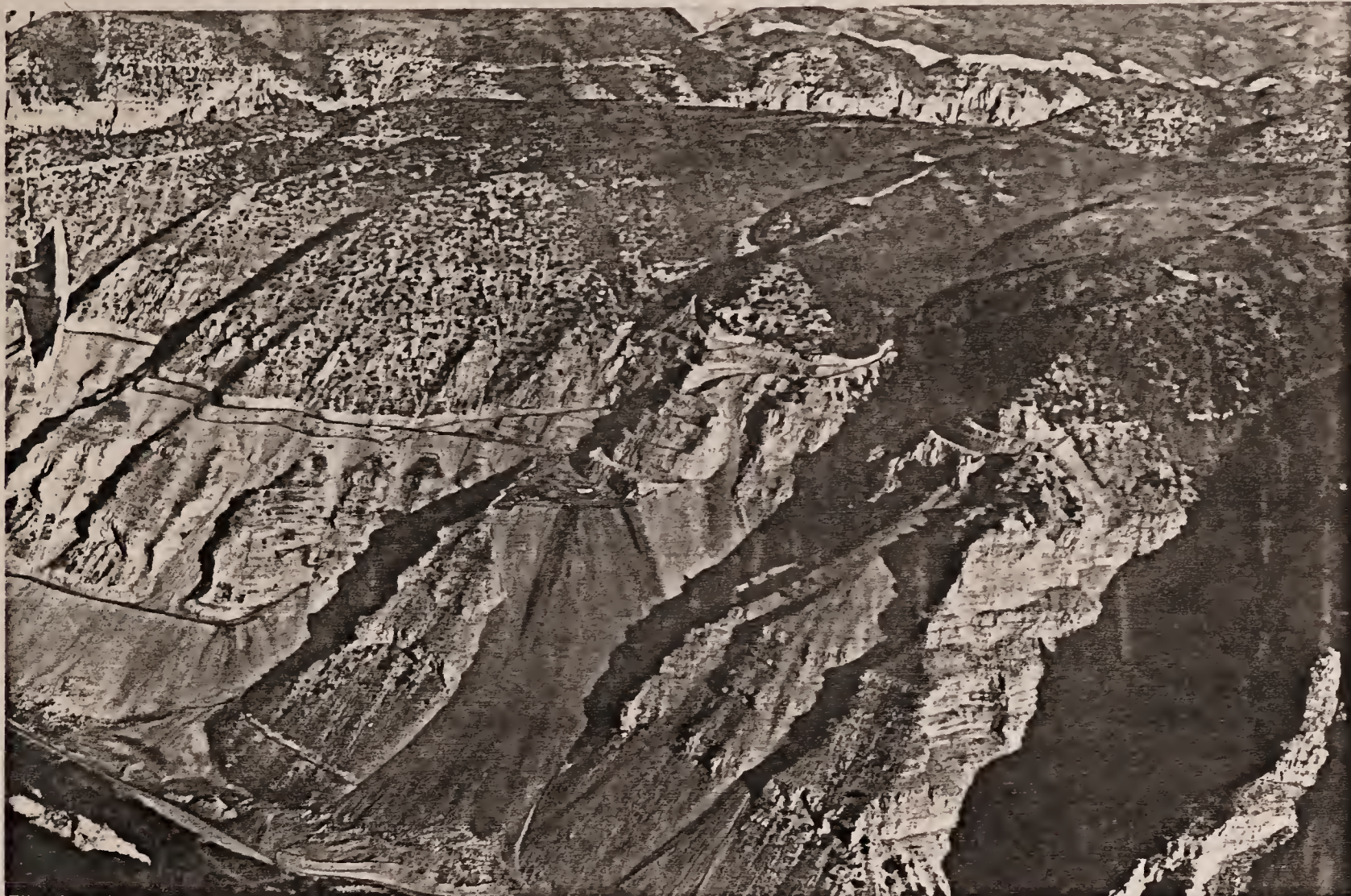
Union 5-acre mine bench on the south side of Long Ridge. Processed shale will be conveyed to valley bottom fill below bench.
