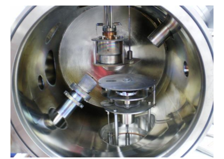
PLD chamber KrF excimer laser \lambda = 248 \text{ nm} (UV)
