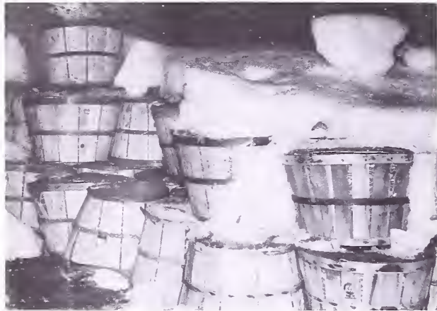
FIGURE 5.—Partly unloaded, longitudinally split load of solid bottom baskets (left background) and continuous-stave baskets (right foreground).
