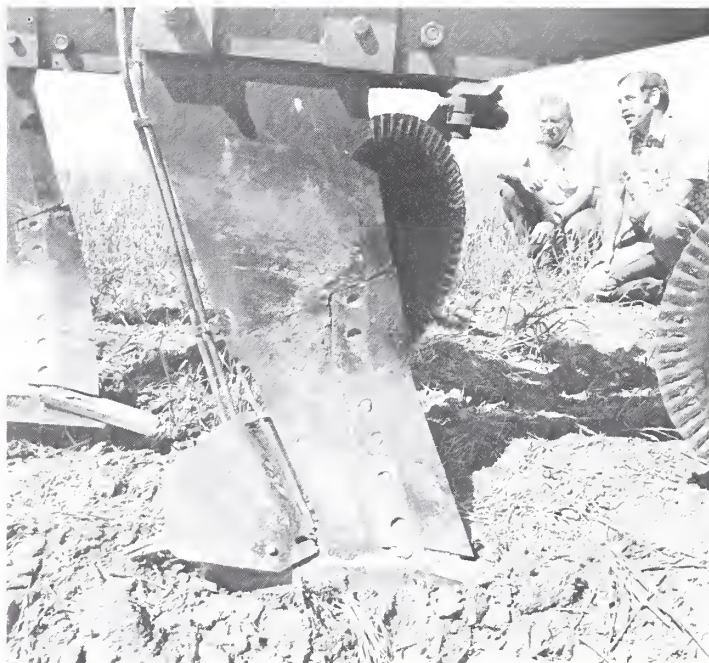
University of Idaho soil physicist John Hammel (right) and ARS microbiologist Lloyd Elliott are testing this British-designed paraplow on the fragile soils of the Palouse. Angled paraplow chisels restore productivity by loosening compacted soil.
