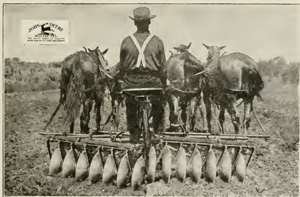
Disc Harrow .. This Implement Is an Insurance Against Loss from Drouth if Used Before and After Deep Plowing
