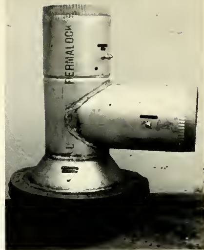
Figure 1.—Nonbreathing valve for Gigi II, constructed of 8 inch stovepipe and containing one quarter inch neoprene foam rubber valve leaflets. Inspiration was from the side-arm, and the inspiratory valve leaf and its supporting ring were slanted so that closure was assisted by gravity.
