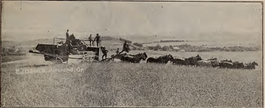
The above cut is from a photograph taken by Prof. Leckenby. It shows a combined harvester at work in Eastern Oregon. It is drawn by thirty-two horses, and cuts, thrashes and sacks the wheat as it goes along
