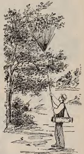
AUTO-SPRAY AT WORK WITH EXTENSION PIPE FOR TALL TREES.
