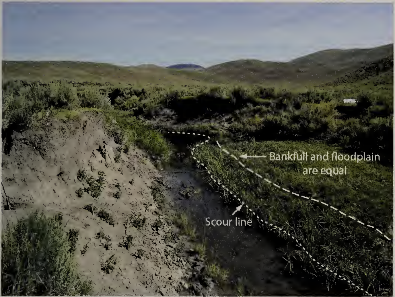
Figure D5. Bankfull and floodplain heights are approximately equal. In this instance, channel incision occurred historically, and a new inset floodplain has formed.
