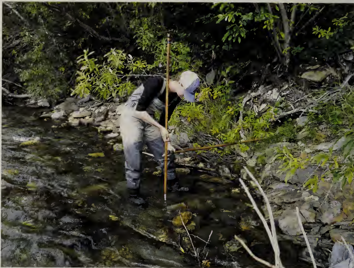
Figure 4. Example of how to use two depth rods to measure bankfull or floodplain height.
