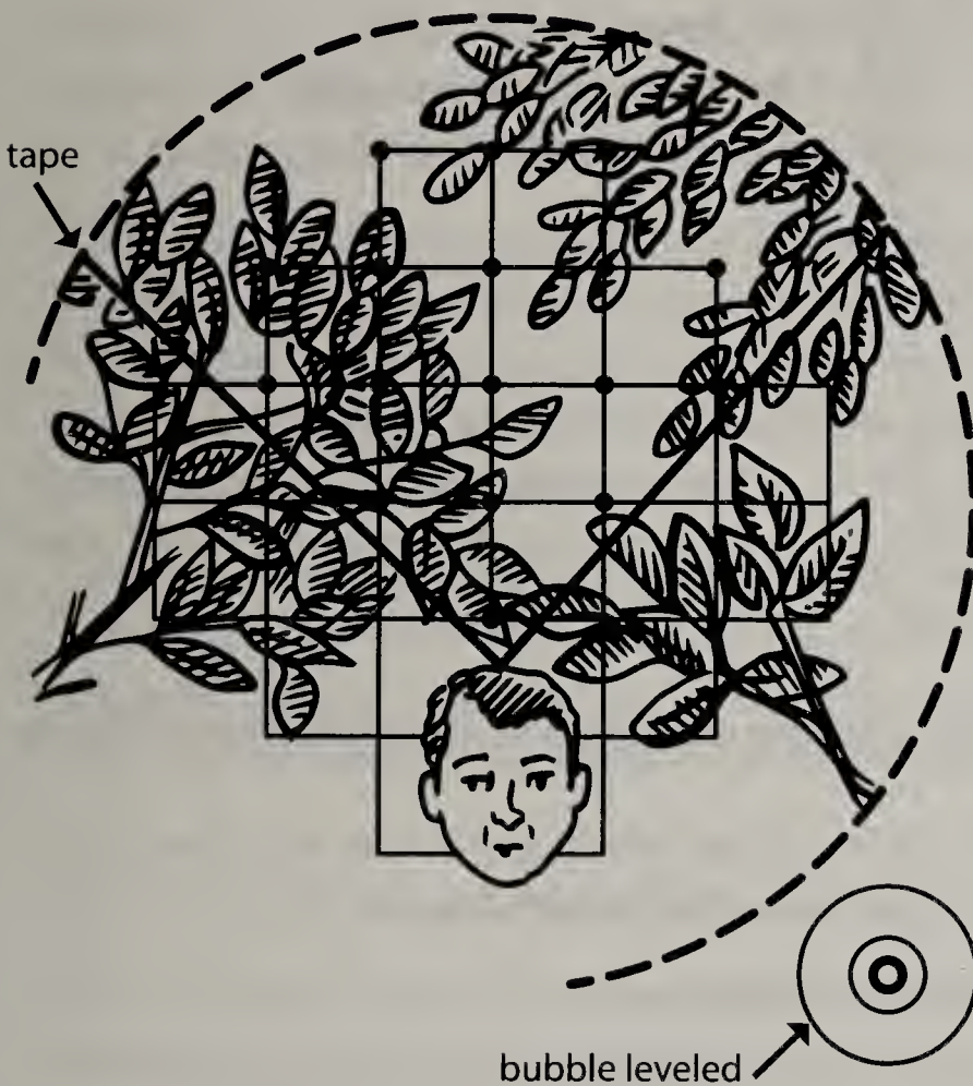
Figure 12. Modified densiometer. Count intersections in the V covered by vegetation or other objects. In this example, the score would be recorded as 10 (USEPA 2009).
