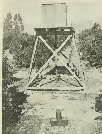
Tower shelter for radiation instruments. It was found that practically all the smoke remained below the top of the shelter and showed practically no influence on the radiation.
