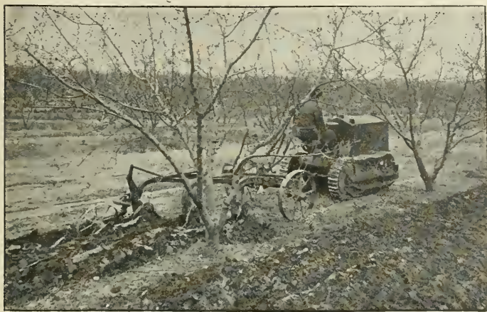
The Small Crawler Tractor, Because of its Compactness and its Smooth Exterior, Handles Implements Right Up to the Bases of the Trees.
