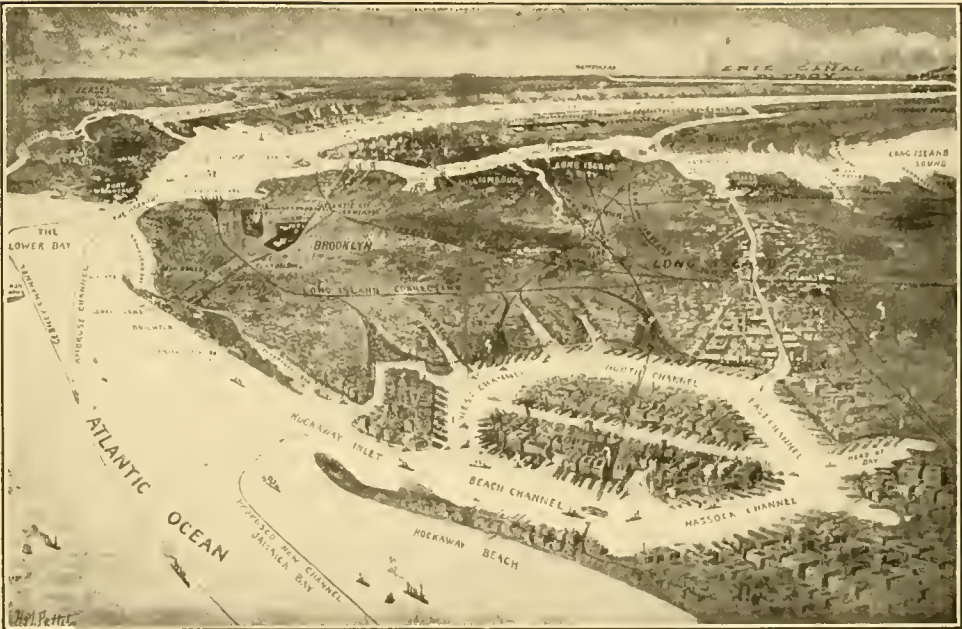
PROPOSED HARBOR IMPROVEMENTS, SHOWING PARTICULARLY THE ROUTE OF THE SUGGESTED CANAL TO CONNECT FLUSHING BAY AND JAMAICA BAY
