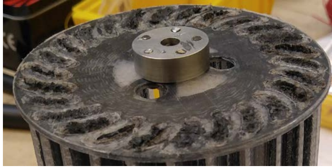
Figure 21. Detail of 3D printed CFF rotor blades bonded to endcap.
