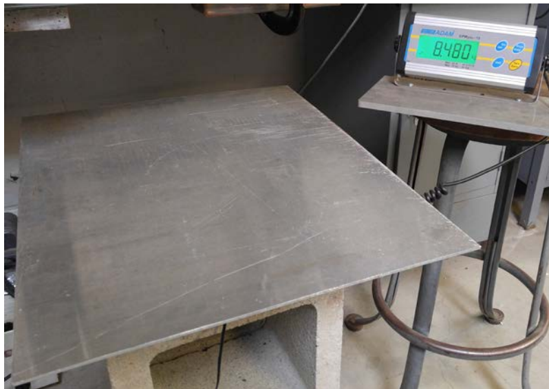
Figure 28. Electronic balance used to measure CFF thrust.
