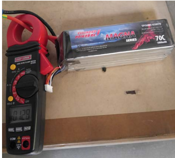
Figure 27. Clamp ammeter measuring current to motor from battery.
