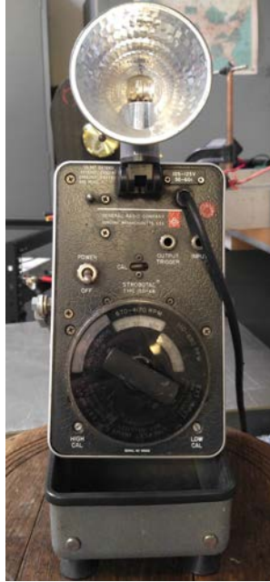
Figure 26. Stroboscope used to measure rotational speed of CFF rotor.
