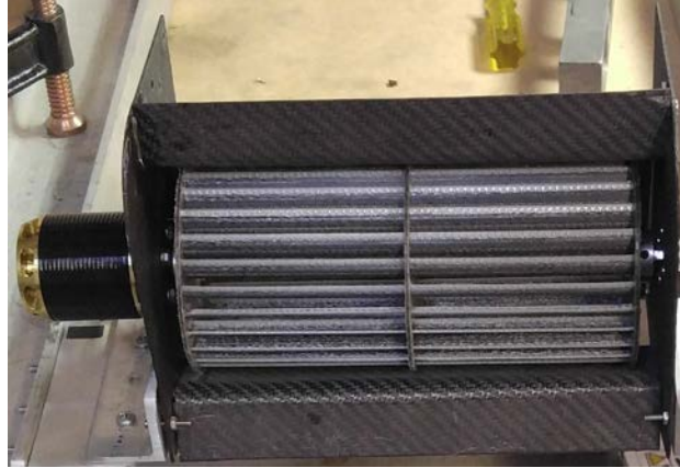
Figure 23. Complete CFF assembly with 3D printed rotor.
