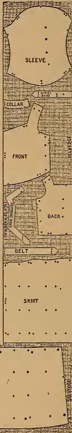
The Most Economical Way of Placing the Pieces of Pattern No. 824 on the Material
