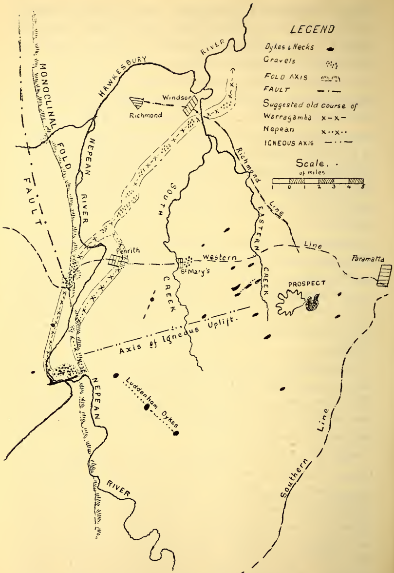
Fig. 2—Map showing the suggested old courses of the Nepean and Warragamba Rivers, and axes of earth movements.
