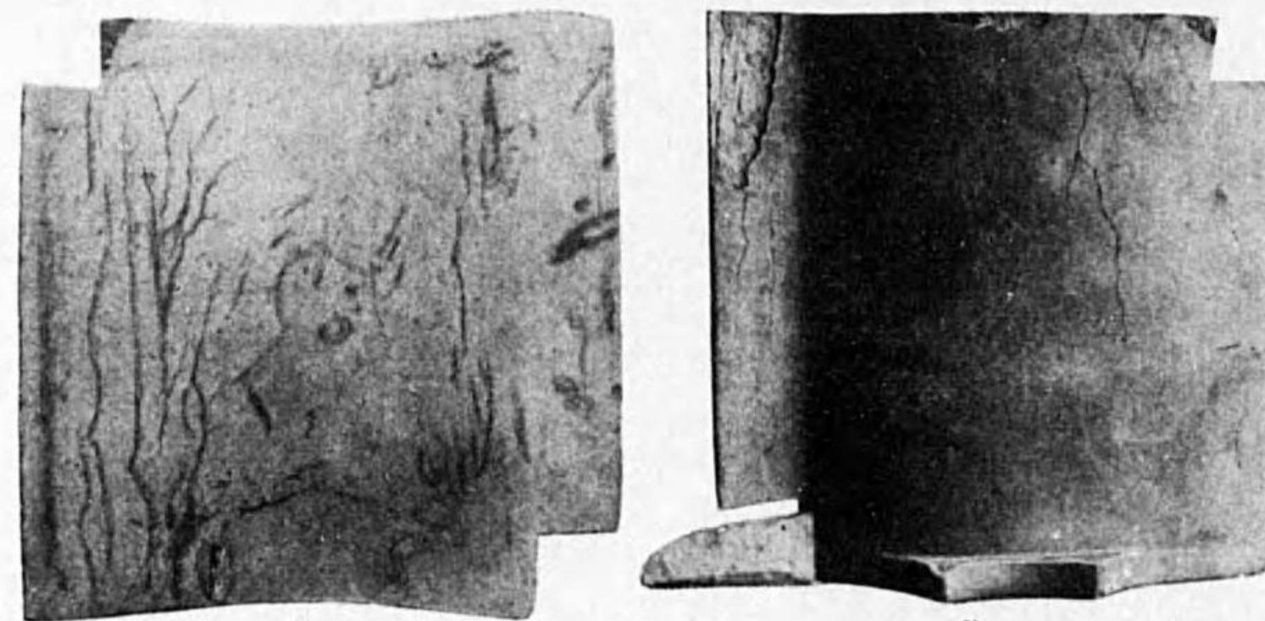
A. B. Fig. 15. Specimen of a roofing tile after freezing and thawing test.
