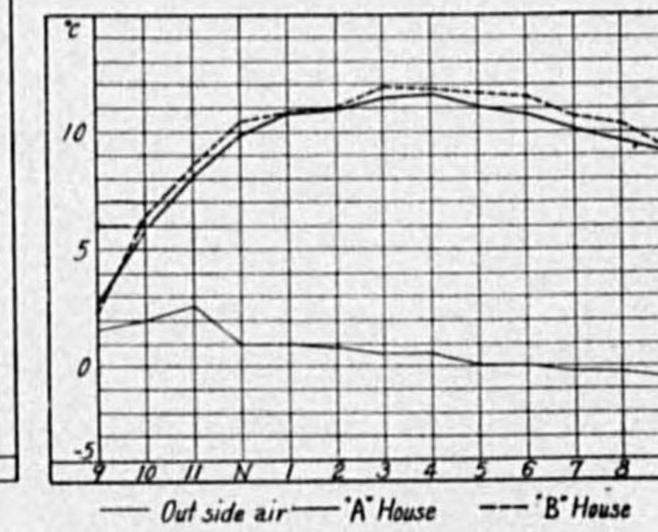
Fig. 15. The comparative results of temperature and humidity in the rooms of A and B houses. (25th Feb.-fine. heating)
