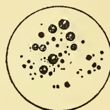
FIG. 1.—SPHERICAL CAVITIES IN ARTIFICIAL RUBY AS SEEN AT ONE TIME (ENLARGED 75 DIAMETERS).
