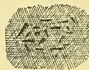
FIG. 4.—CUNEIFORM CRYSTALS IN RUBY AND SAPPHIRE (ENLARGED 200 DIAMETERS).
