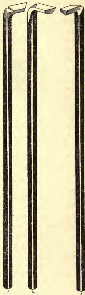
FIG. 4.—Different views of special tool for cutting cell (Fig. 3 B) from cylinder (Fig. 3 A).
