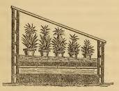
It is described as a very useful and most desirable structure for the growth of the pine apple, with a hollow wall, recommended by all garden architects in preference to a solid wall—the heat or cold being not so readily conducted as through a solid mass of masonry. Mr. Rendle might have added, that hollow walls are also much drier. (Rendle's Treatise on the Tank System).
