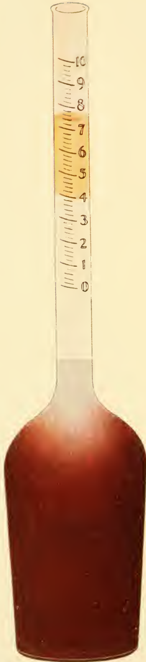
Babcock Flask, Showing Fat in Neck (after Harrington)
