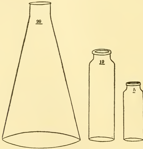
Flasks and vials for quantitative bacteriological analysis.
