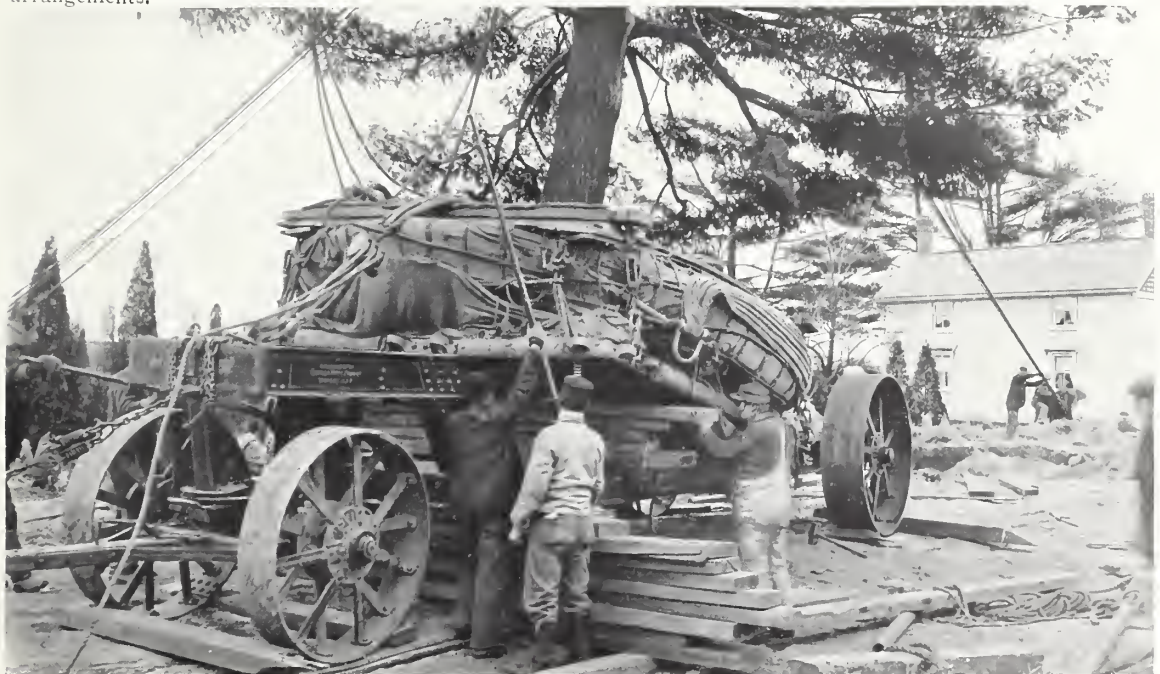
Tree Mover No. 21, all steel. Estimated capacity 30 tons. On the mover is the Pine, illustrated on back cover. Whatever the nature of the work may be, we have apparatus uniquely adapted for it and what may be of still greater importance, knowledge as to what may or may not be best in tree moving.
