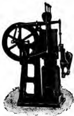
Fig. 78. Ericsson hot-air engine.
