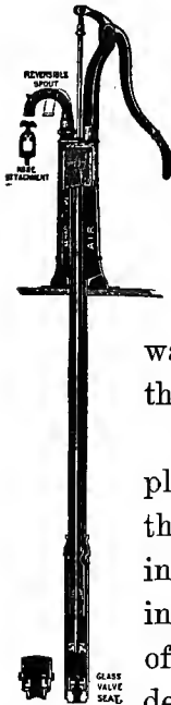
Fig. 38. Well force pump.
