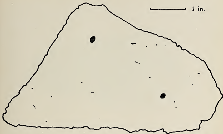
FIGURE 4. Distribution of troilite in the etched face shown in Fig. 3. The smaller particles were located by means of a sulfur print.
