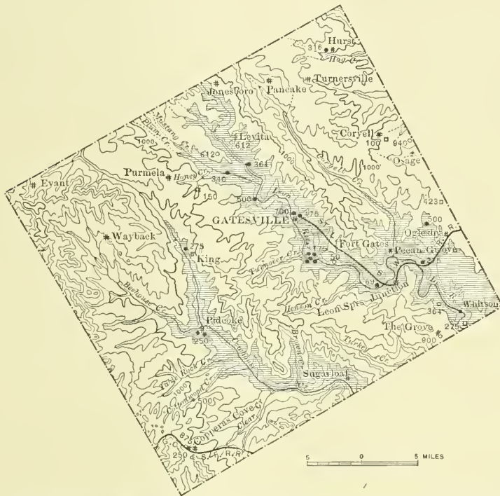
FIG. 56.—Artesian map of Coryell County, Texas. Shaded portion indicates area where flowing wells are likely to be obtained; ●, flowing wells from Trinity reservoir; ○, non-flowing wells from Trinity reservoir; □, non-flowing wells from Paluxy reservoir; figures indicate depth of wells in feet.
