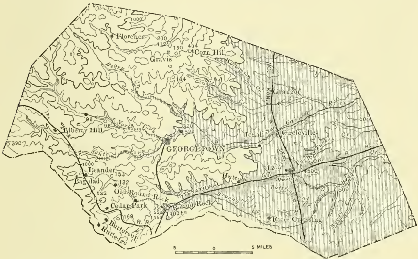
FIG. 62.—Artesian map of Williamson County, Texas. Shaded portion indicates area where flowing wells may be obtained; ●, flowing wells from Trinity reservoir; ○, nonflowing wells from Trinity reservoir; figures indicate depths of wells in feet.
