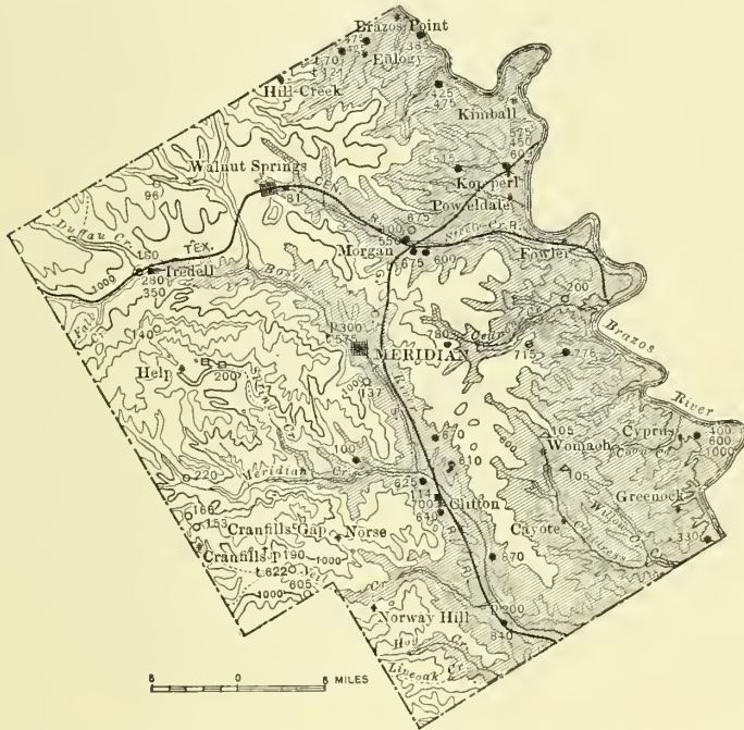
FIG. 54.—Artesian map of Bosque County, Texas. Shaded portion indicates area where flowing wells can be obtained from the Basement Trinity reservoir; ●, flowing wells from Trinity reservoir; ○, nonflowing wells from Trinity reservoir; figures indicate depths of wells in feet.
