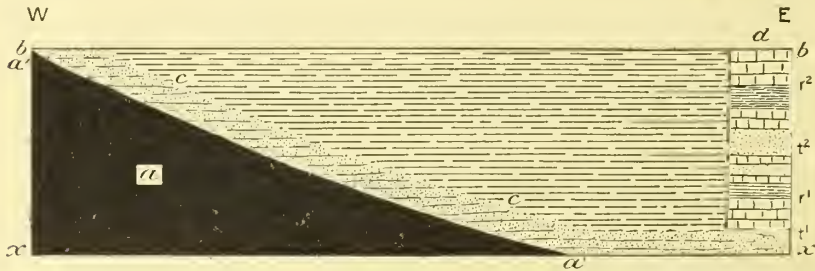
FIG. 8.—Diagram showing change in nature of sediments of Glen Rose beds. a , the Paleozoic floor; a' a' , the deposition surface; c c , the Basement sands; d , columnar section; x x , sea level at beginning of Cretaceous epoch; b b , sea level at close of Trinity stage. (For explanation of other symbols see Pl. XVI, p. 110.)
