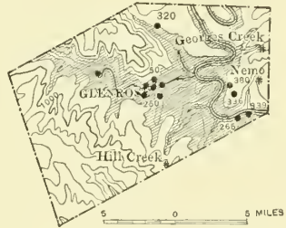
FIG. 53.—Artesian map of Somervell County, Texas. Shaded portion indicates area where flowing wells should be obtained from the Basement Trinity reservoir; ●, flowing wells from Trinity reservoir; figures indicate depth of wells in feet.
