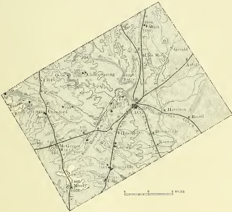
FIG. 67.—Artesian map of McLennan County, Texas. Shaded portion indicates area of possible flow from the Burnet-Trinity reservoirs; ●, flowing wells from Trinity reservoir; ○, nonflowing wells from Trinity reservoir; ■, flowing wells from Paluxy reservoir; □, nonflowing wells from Paluxy reservoir; △, nonflowing wells from Fredericksburg reservoir; figures indicate depths of wells in feet.
