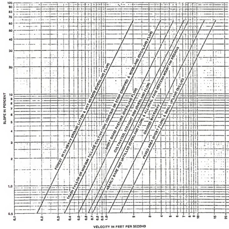
Fig. 2—Velocities for upland method of estimating  $T_c$
