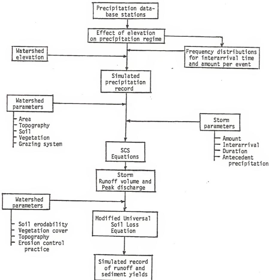
Fig. 3 Flow chart of simulation process.
