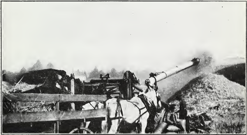
FIG. 2.—SAME MACHINE THRESHING WITH 14 PER CENT SMUT (ESTIMATED) IN CROP, SHOWING BLACKER SMUT-DUST CLOUD COMING FROM BLOWER PIPE.
