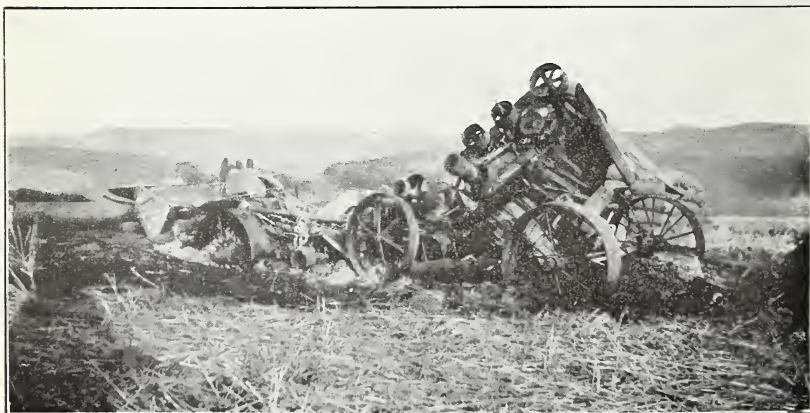
FIG. 3.—WOODEN MACHINE COMPLETELY DESTROYED BY SMUT EXPLOSION AND FIRE IN PACIFIC NORTHWEST.
