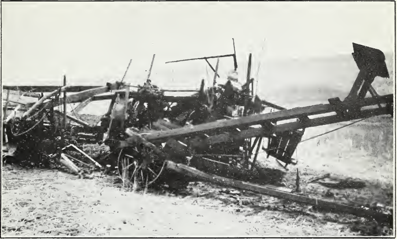
FIG. 1.—COMBINE MACHINE AFTER SMUT EXPLOSION AND FIRE, IN EASTERN WASHINGTON.
