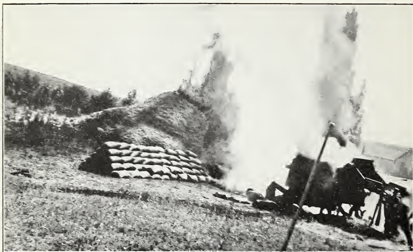
FIG. 1.—SMUT-DUST EXPLOSION IN THRESHING MACHINE IN EASTERN WASHINGTON. PHOTOGRAPH WAS TAKEN AT TIME EXPLOSION AND FIRE OCCURRED.
