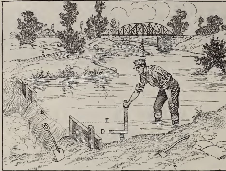
Courtesy Barnard and Lees Co., Mobile, Illinois Locating a Farm Power—Measuring Stream Discharge With a Weir
