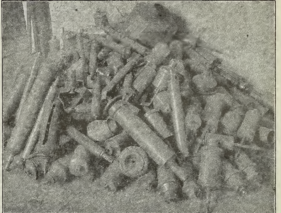
(A sample pile of scrapped competitive separator bowls—the frames being broken up in the field to save freight on same.)
