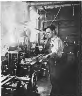
What's wrong with this picture? It represents a typical case which the Human Auditor uncovers. Everything in this corner "passes" the auditor's inspection—light, ventilation convenience. But there is something—something which has escaped the employer's attention—something which may be fatal. The employee is a casting-room operator in a print shop. He should not be allowed to EAT in the room.
